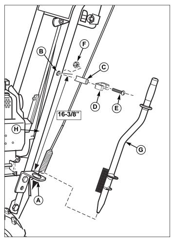
Figure 6. Mounting Clean-Out Tool (Tube Handle)
